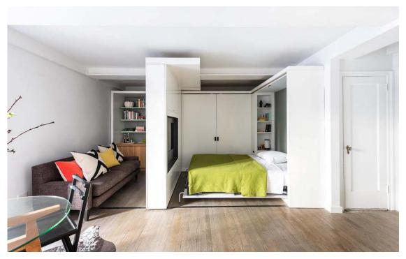
When the wall is in its closed daytime position, the space has a generous living room. When the wall is opened, it creates a space that can be used as a changing or bed room, depending on whether the queen-sized wall bed is lowered. The interior wall that is perpendicular to the moving wall is lined with a volume that contains a desk on one side and a wardrobe on the other.
