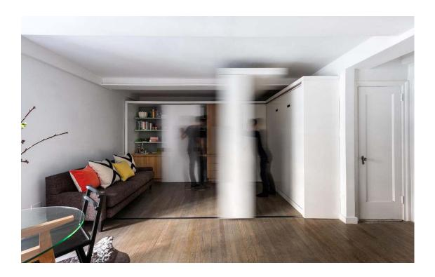
Similar to the LifeEdited apartment, "5 to 1" incorporates a moving wall to provide additional "rooms" for the 390 sq ft Manhattan apartment. The wall, which was custom fabricated by **Trak-Kit**, is fully motorized and has power as well as cable for television and audio. The wall also houses networking components and audiovisual equipment, which includes a TV that rotates 180 degrees to face either side of the wall.
